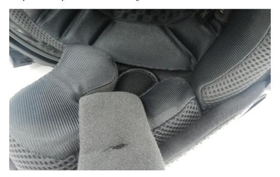
2. Applying the other speaker to ear pocket inside helmet on left side and applying the microphone support also on the left inner liner of the helmet.
