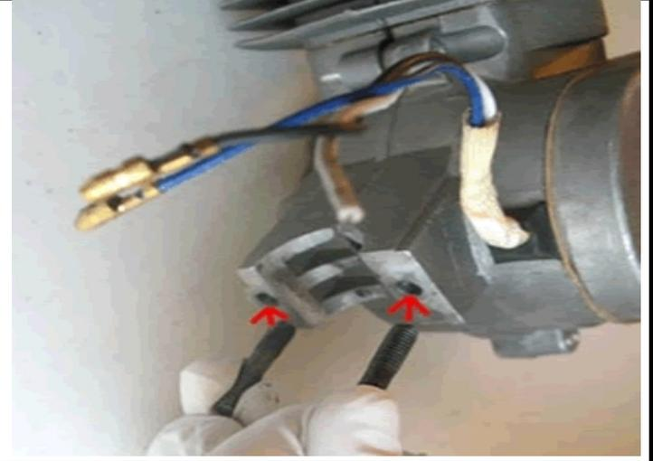
Bicycle frame adapter installed to the engine
